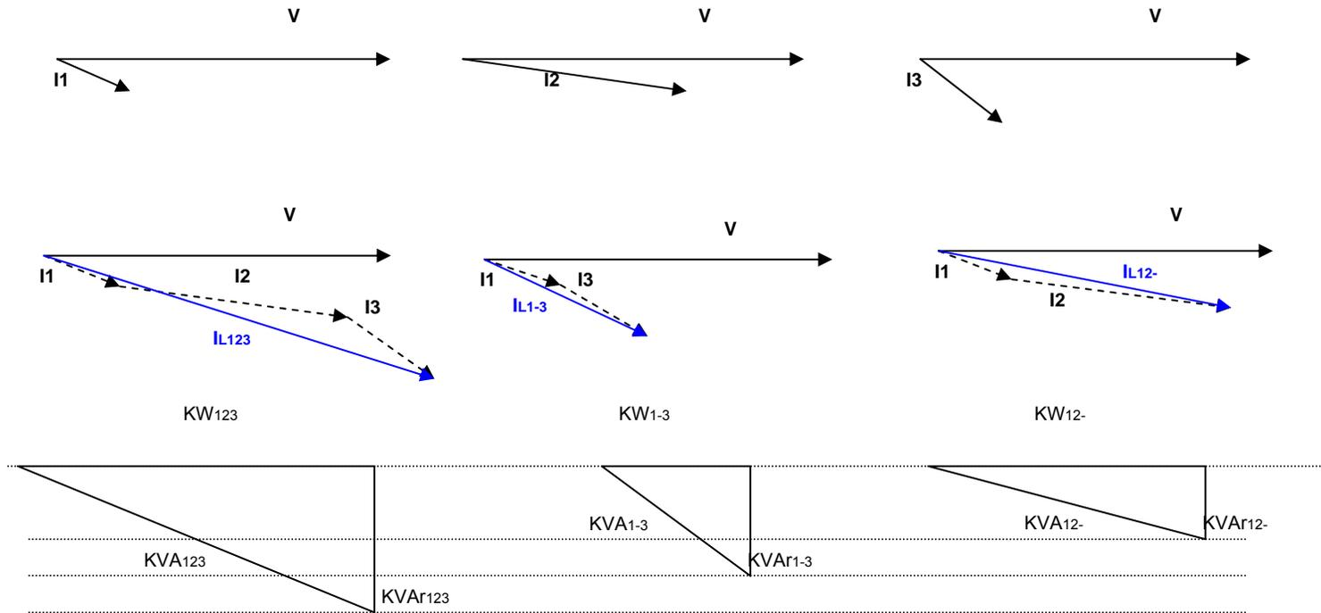
The situation above shows that variable kVAR compensation is needed for various loading conditions.
