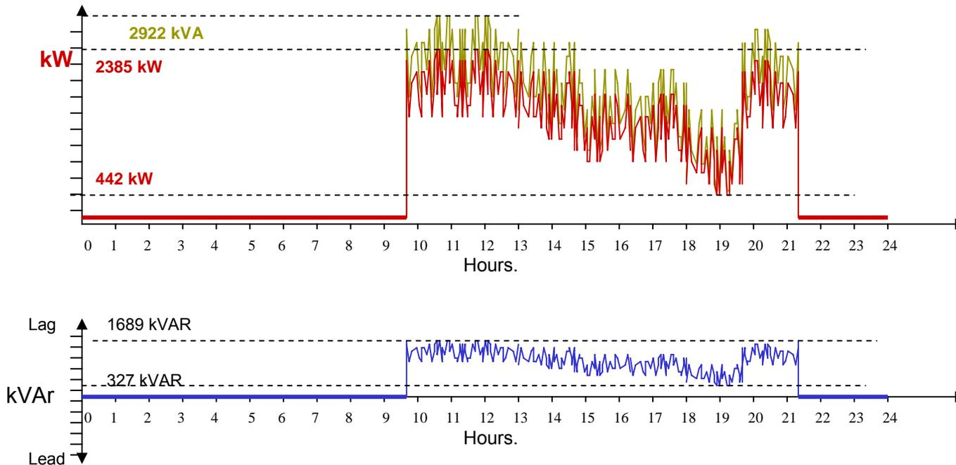
The above plot is on one of the agricultural feeder. In-operation hours are 11:30 Hrs. The plot is taken when there is no capacitive compensation provided on the feeder. Total number of APFC systems per feeder provided 45Nos.(various ratings)
